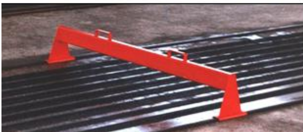
Safety Bars placed at regular intervals along a concrete production bed
