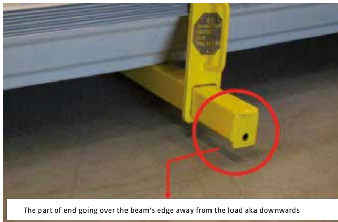
Figure 10. The harnesses at the end of the beam show in which direction the beam must be located for lifting
