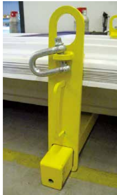
Figure 14. Fastening of a lifting shackle to the leveller.
