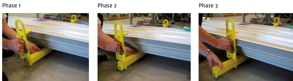
Figure 11. Placing the beam part under the load in parts
