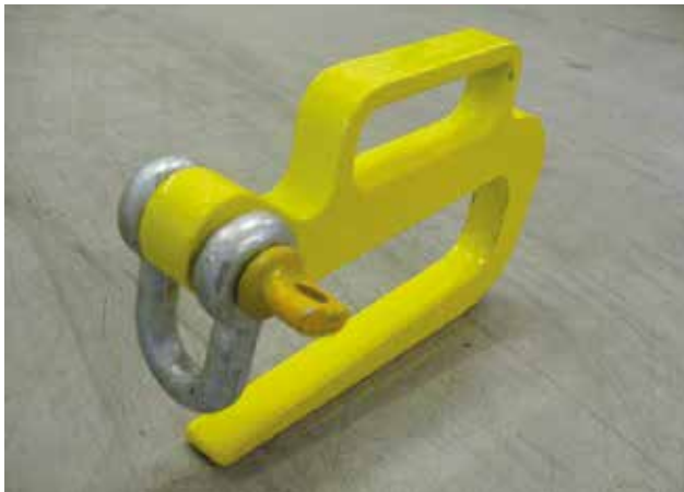
Figure 13. Fastening of a lifting shackle to the hook.
