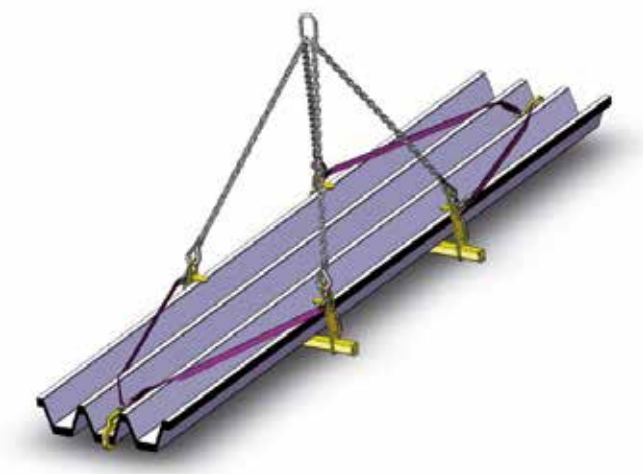
Figure 21. Mounted lifting tool with load and chain threads.
