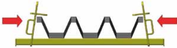
Figure 12. The levellers must be pushed as close to the load as possible.
