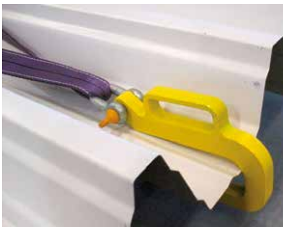
Figure 15. Fixing the lifting belt to the lifting shackles.
