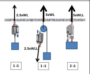
If the fixing of the unit must be in a dangerous place for the operator, the safety precautions provided for by the work's regulation must be taken to exclude any risk uncontrolled in this operation. It is perhaps better in this case to implement the hoisting cable into the device before the anchoring operation.
