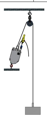
The resistance of the pulley and its anchorage must be calculated for a double effort of the lifted load.
