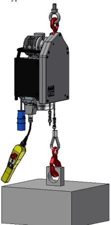
This winch is designed for the lifting and traction of loads. It is intended for professionals involved for work, such as in an elevator shaft or on building facades. The winch uses one steel cable (hoisting cable).
