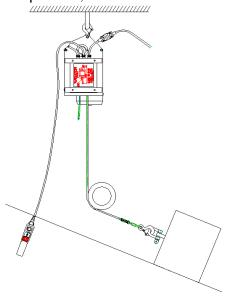
This case requires a deflection pulley anchored to a fixed point.
