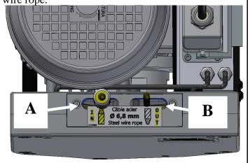
PS: a second stopper is provided to stop the descent; position the spring on the side of the winch:
