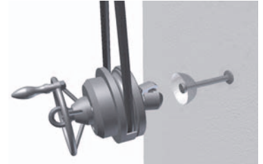
Press tightly onto the anchor head.
