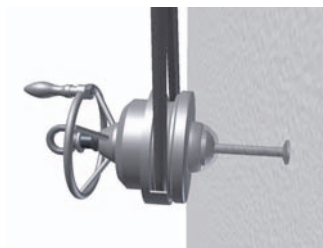
The handwheel is turned until the turning and lifting link sits tightly against the concrete.
